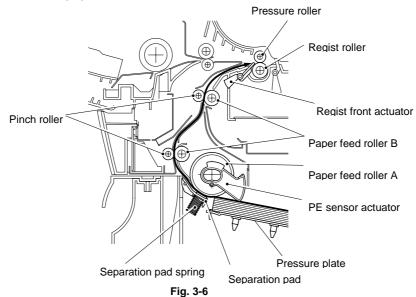
The paper is gripped between the paper feed roller A and the separation pad and separated into individual sheets.
