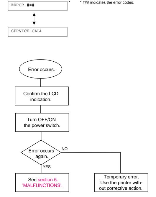
Holding down the – switch and the **Set** switch at the same time while the error messages display will cause the type of the error appears on the LCD display.
