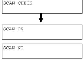
The automatic correction of twin laser has been finished correctly.
