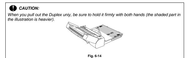
(4). Pull out the jammed paper from inside the Duplex unit.
