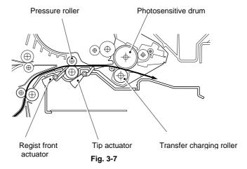
The tip actuator in the path from the pressure roller to the transfer charging roller controls the first print position on the paper.
