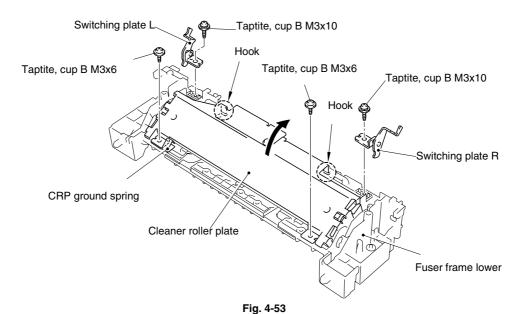
(21) Turn over the cleaner roller ASSY, remove the edge of the cleaner roller ASSY AMs as shown in the figure below while pushing down the cleaner roller bearings.
