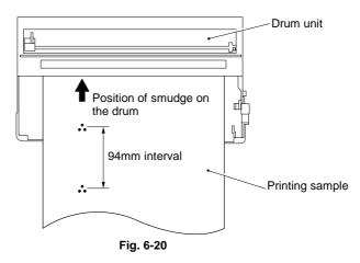
(2) Turn the drum gear by hand while looking at the surface of the photosensitive drum. Be sure to turn the drum gear in the direction of an arrow.
